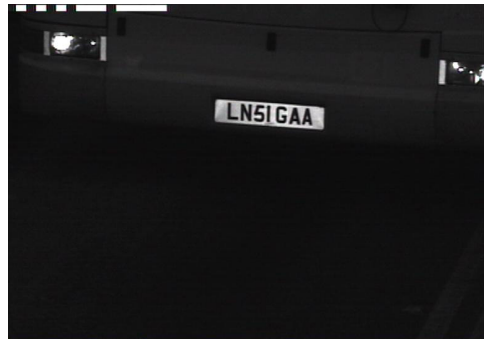
ANPR Image with Speed Barcode
